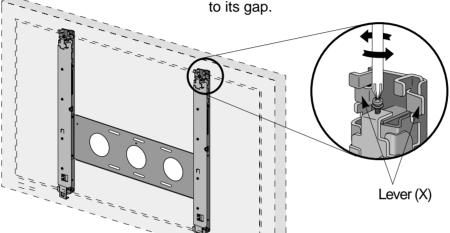
As pictured below, pull and adjust the lever (X) to fit your desired viewing angle.
